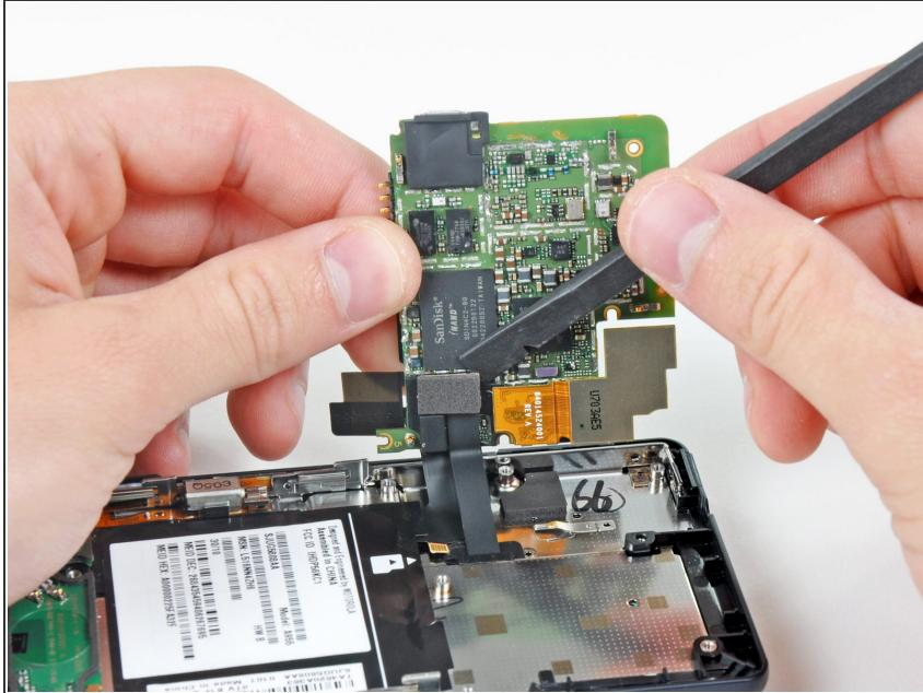
**i** Carefully lift the motherboard from the front case and lay it next to the Droid 2, minding the keypad connector that is still attached.
