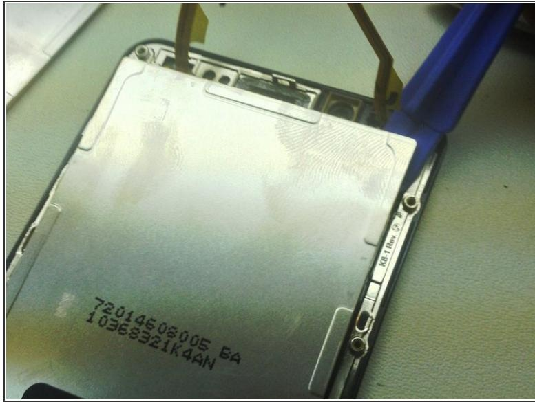
**⚠** Carefully peel the two flex cables from the back housing of the LCD. Be exceptionally careful during this process, as those flex cables can be easily ripped.
