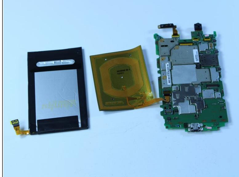
**⚠** Carefully peel back the orange adhesive from the battery. Make sure to remove all the adhesive attaching the battery to the motherboard.
