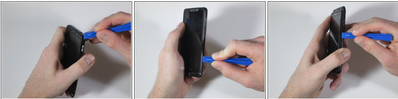
**⚠** When you detach the front from the back, don't pull the two pieces entirely apart. There is a flat orange wire that connects the two pieces that will be disconnected in the next step.
