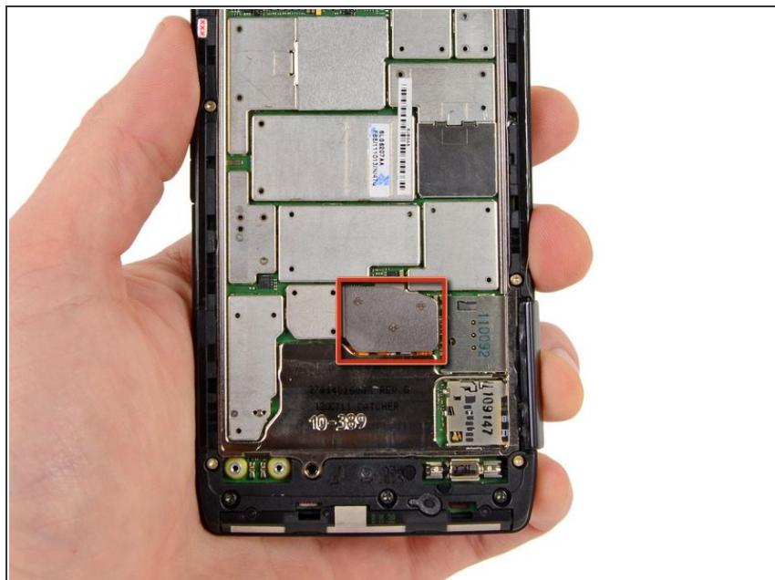
*(i)* There is a small metal shield that covers the display assembly cable connectors on the motherboard. This shield is held in place by a few small clips that attach to the surrounding EMI shields.
