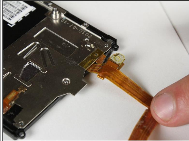
! Carefully pull the long orange cable away from the device.
