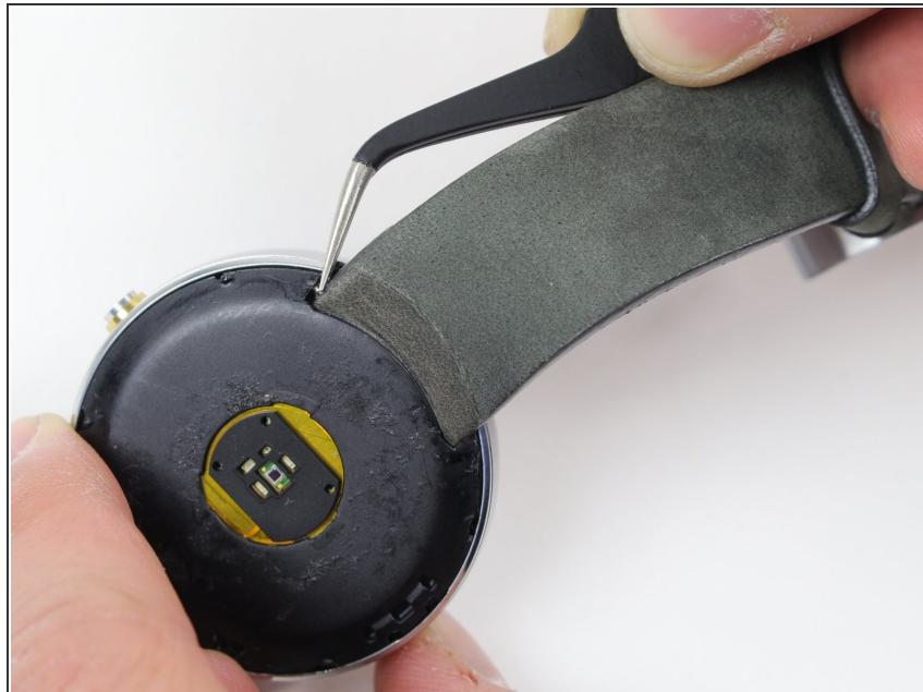
⚠ Take care not to lose the spring-loaded pin when removing the strap.
