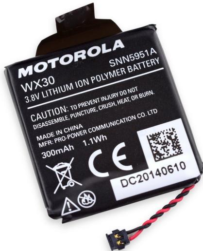
ⓘ There's something [afoot](#), because Motorola has marketed the Moto 360 as having a 320 mAh capacity battery, but the battery is clearly marked as 300 mAh.
