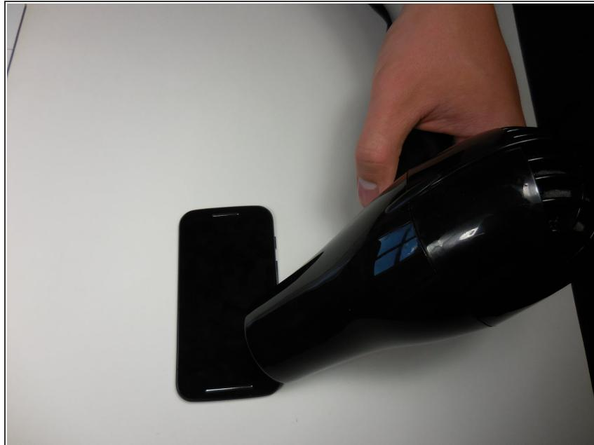
*(i)* To put the new screen on, press the new screen and digitizer into place, and then reapply heat to adhere the new screen.
