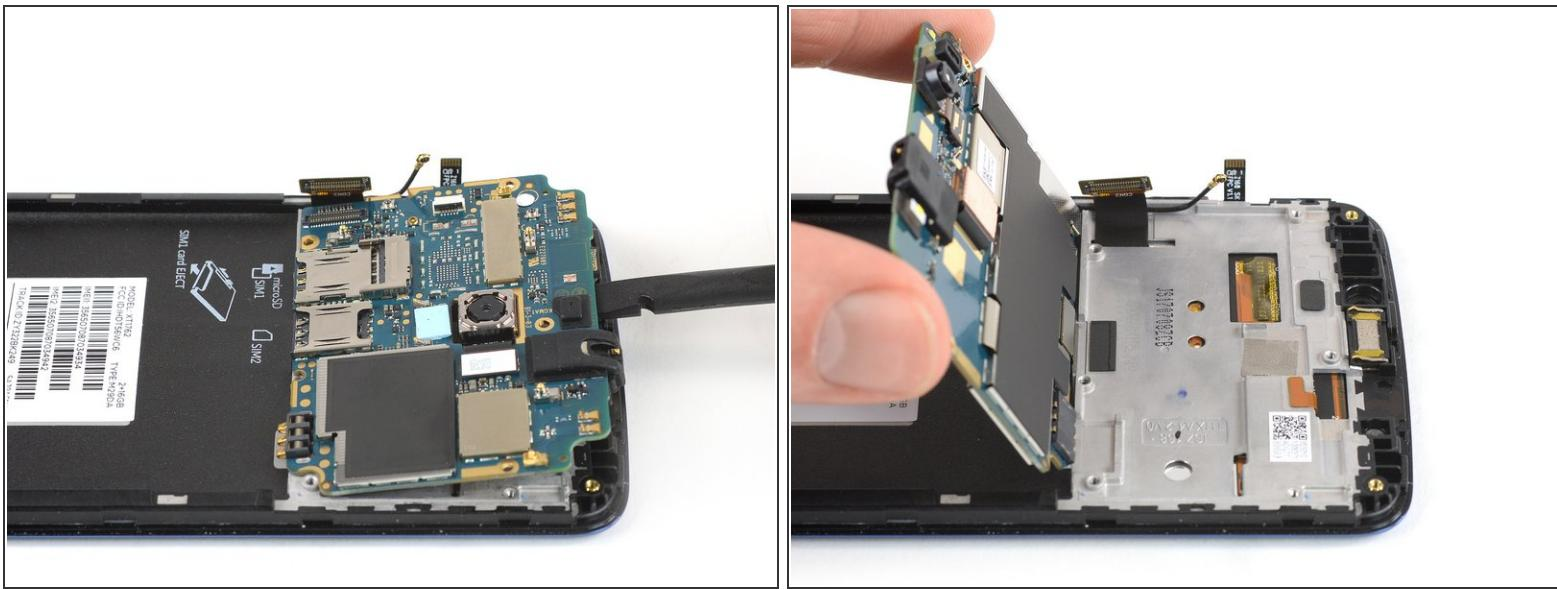
**⚠** Don't try to remove the motherboard all the way yet. The interconnect flex cable is still connected to its rear side.
