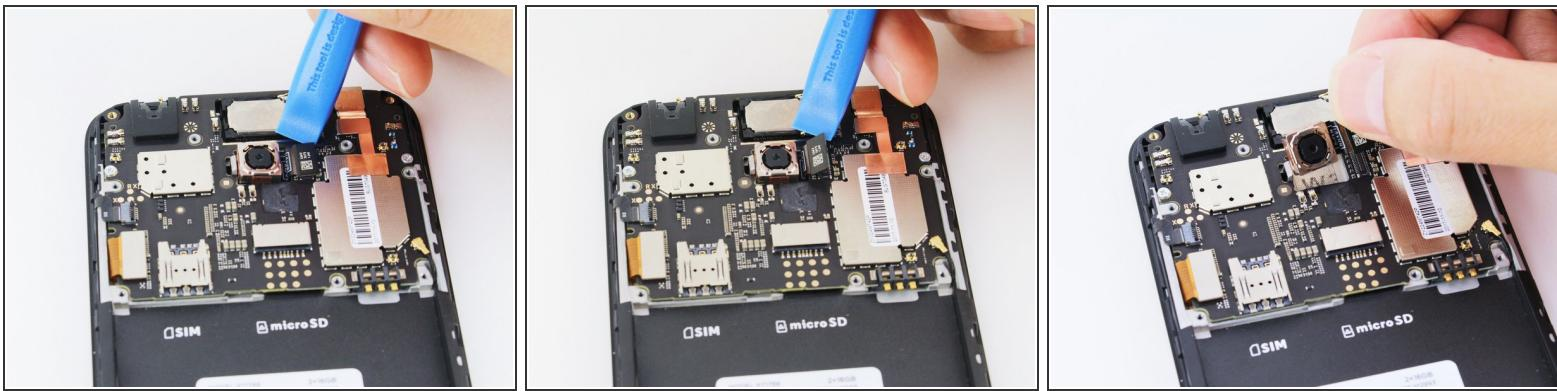
*(i)* This step can be skipped if you are only removing the front-facing camera. For all other repairs, continue as follows.
