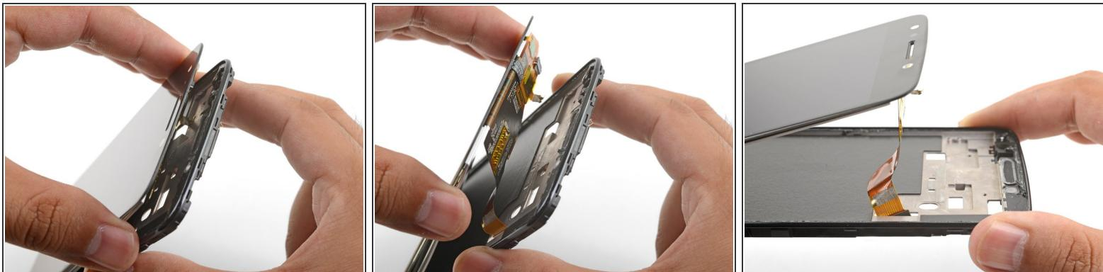
*(i)* The screen cable is still adhered to the frame.
