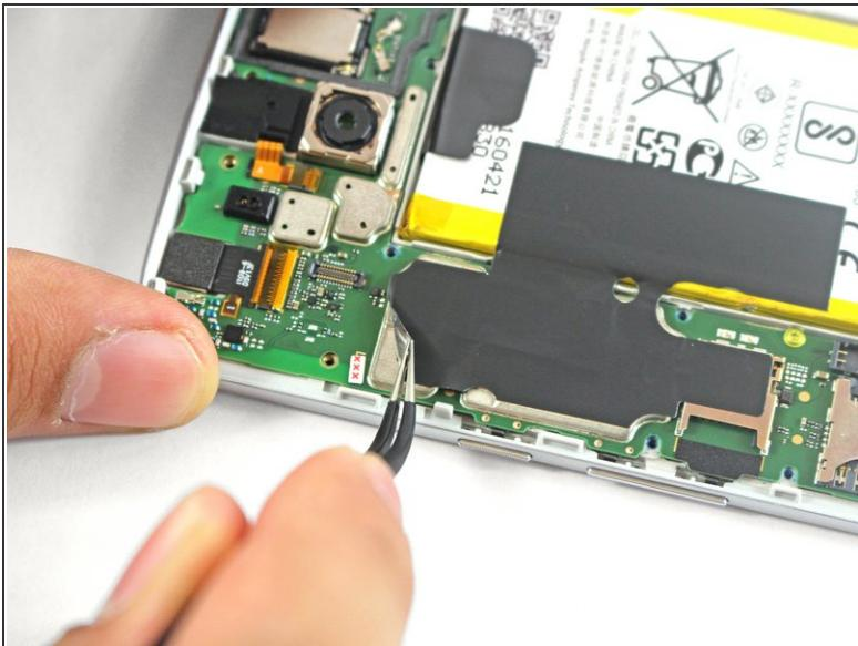
**⚠** Be very careful not to puncture the battery with any sharp tools. A damaged lithium-ion battery can catch fire and/or explode.
