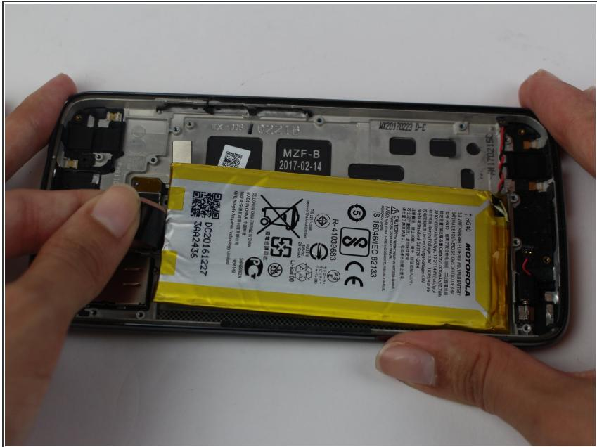
**⚠** Do not use the heat gun to try and remove the battery. Heating a lithium-ion battery can cause it to catch fire.
