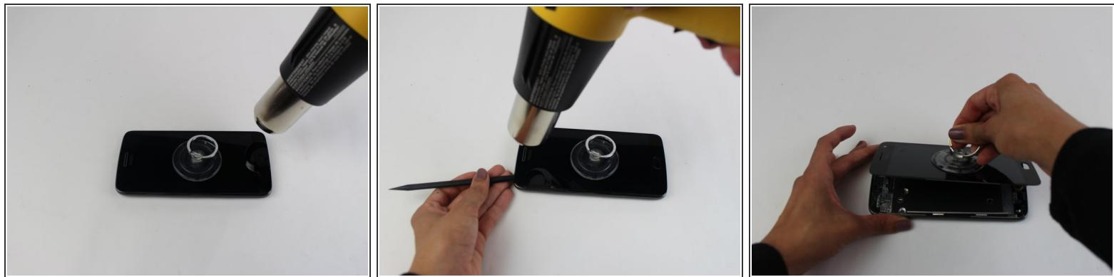
**⚠** The screen is likely to crack as you pry it up. You should not complete this step unless you have a replacement screen available.
