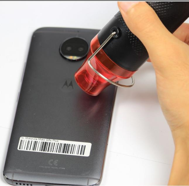
**⚠** Heating up the battery excessively could cause the battery to ignite
