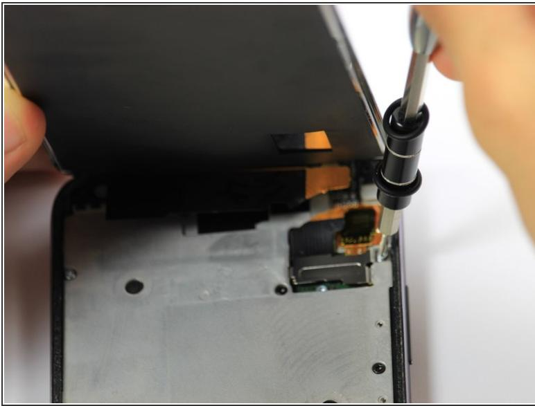
**⚠** The cables at the top of the device are fragile. If you are using this guide as a prerequisite for replacing another part, be careful not to tear the cables while lifting the screen.
