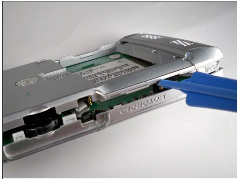
**⚠** Wedge the plastic opening tool in between the top and bottom cases. This may require a little or a lot of force so be careful.
