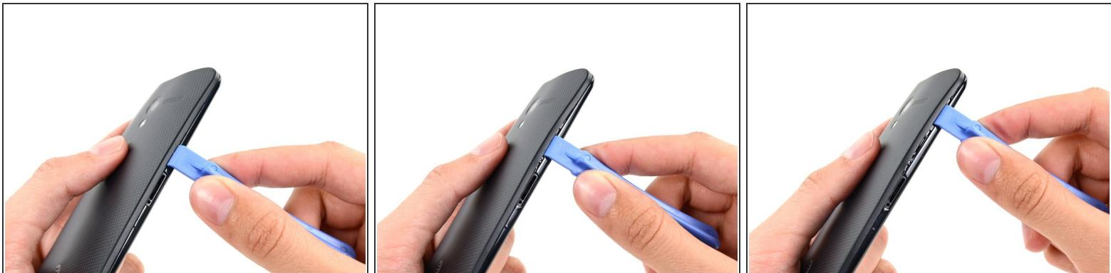
*(i)* In the following steps you will be releasing the clips holding the phone's cases together. However, the back case is also secured with an adhesive pad. After separating the clips you will use an iOpener to allow the case to fully open. **Do not** attempt to fully open the phone before loosening the adhesive.
