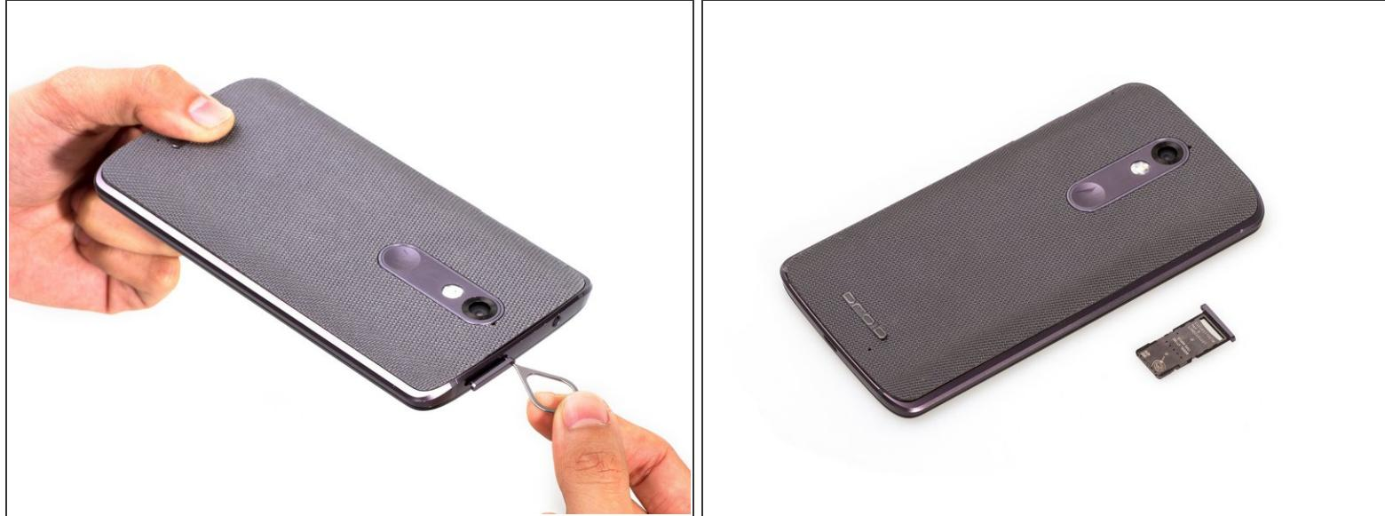
⚠ Remove it or it will be a barrier to remove motherboard.
