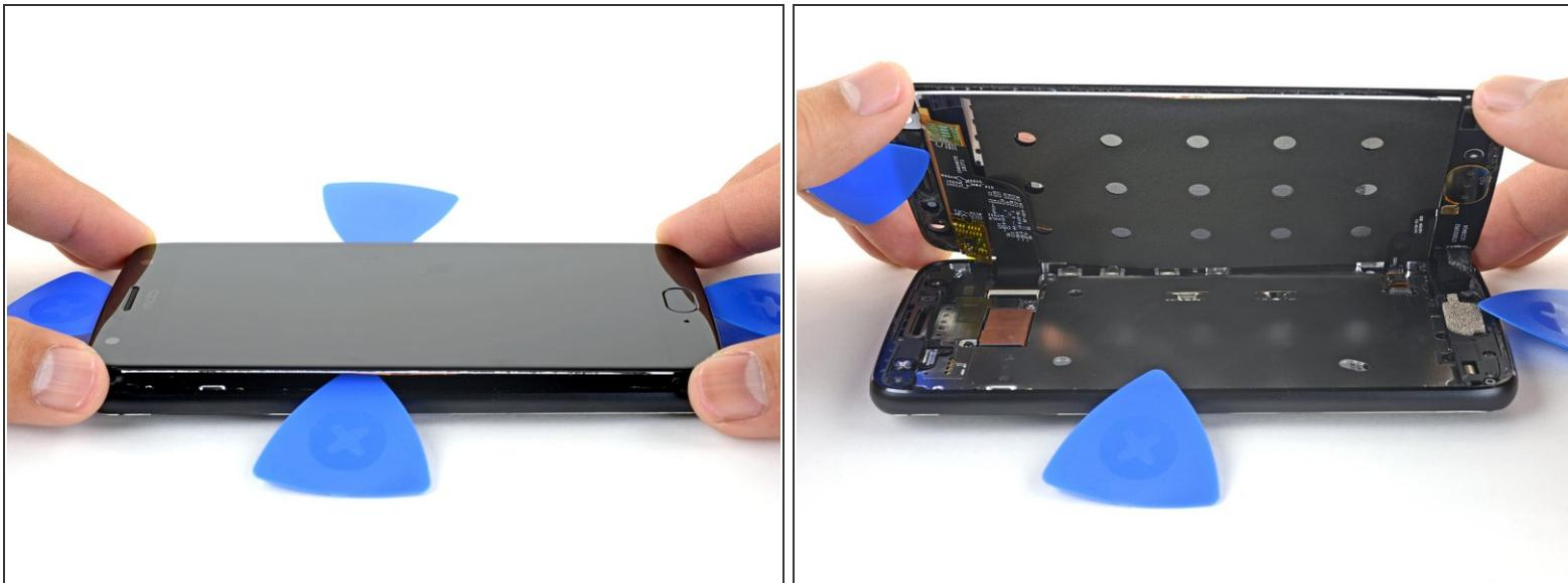
! Do not try to remove the screen yet—it is still attached to the phone by delicate flex cables.
