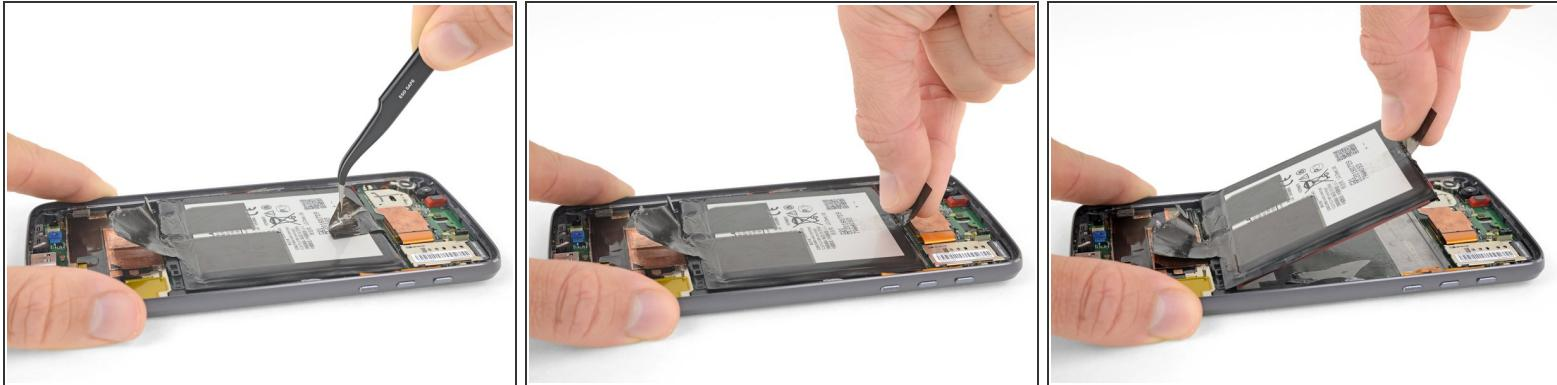
**⚠** In the following steps you will only lift the battery, **do not completely remove it**—it's still connected to the motherboard.
