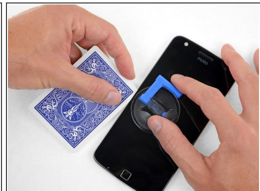
ⓘ In the following steps, you will separate the display assembly from the Moto Z Play's chassis.
