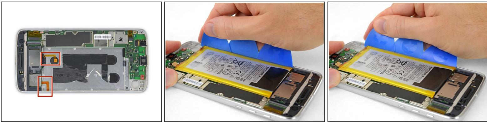
**⚠** When using tools to pry up the battery, be careful not to damage the two orange flex cables hidden underneath the battery's top edge.
