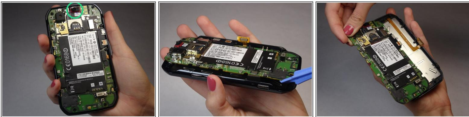
**⚠** Be careful when removing motherboard. Earpiece is connected with small wires and adhesive. Use thin metal tool to pry off before removing motherboard.
