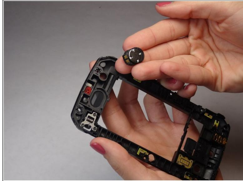
⚠ The speaker is attached to the midframe with adhesive. Remove carefully.
