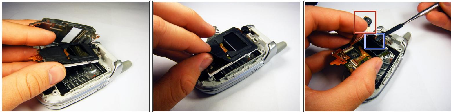
**⚠** Carefully remove the protective cover from the circuitry
