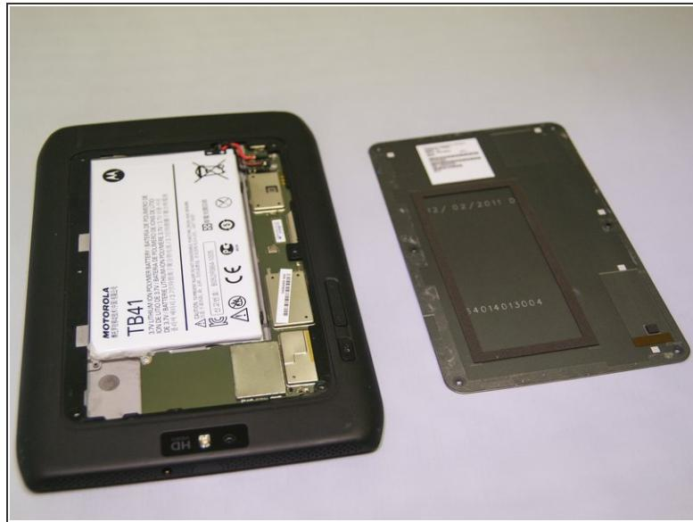
**⚠** There is adhesive attached to the underside of the back panel. Gradually lift panel to avoid bending it out of shape.
