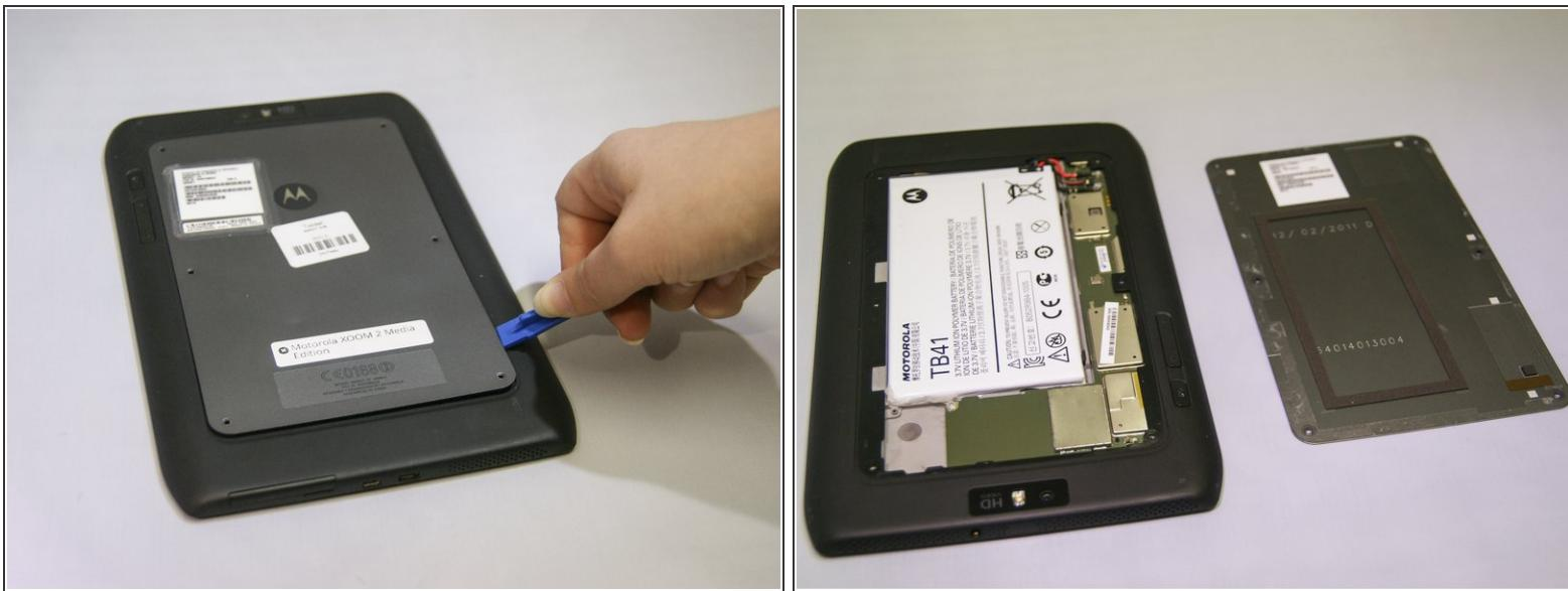
**⚠** There is adhesive attached to the underside of the back panel. Gradually lift the panel to avoid bending it out of shape.
