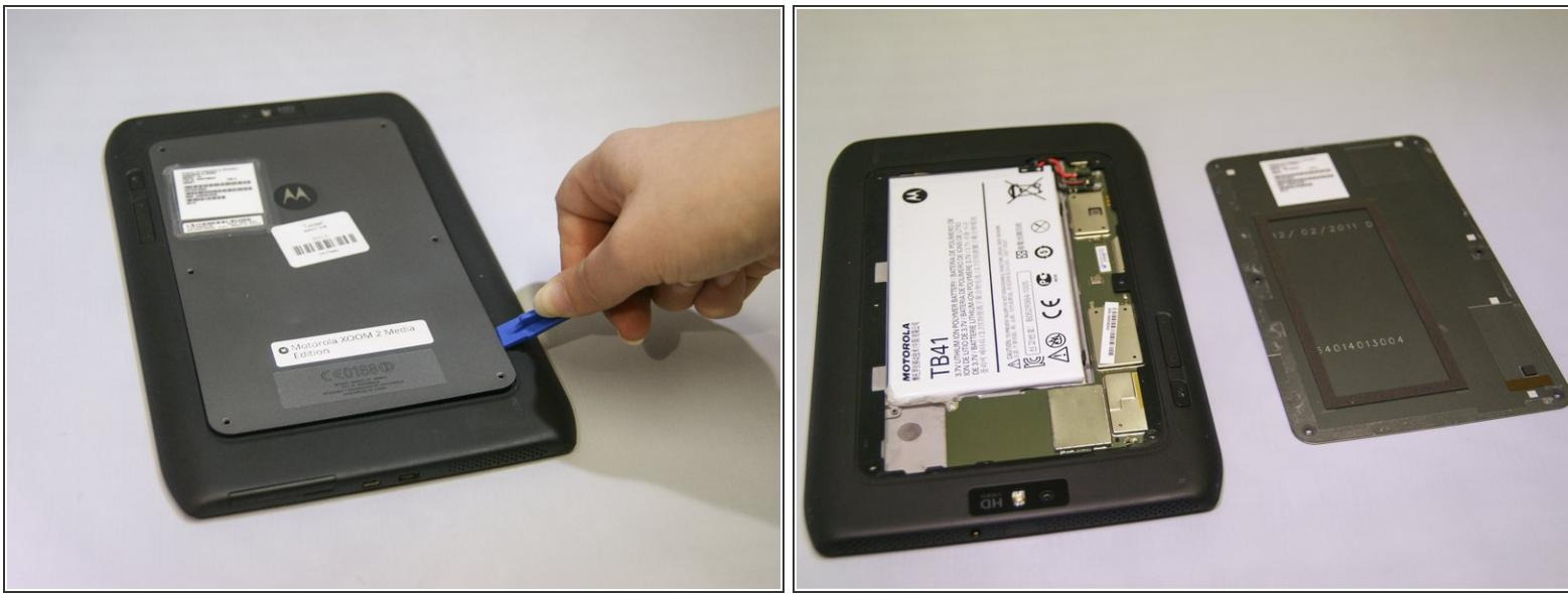
**⚠** There is adhesive attached to the underside of the back panel. Gradually lift the panel to avoid bending it out of shape.
