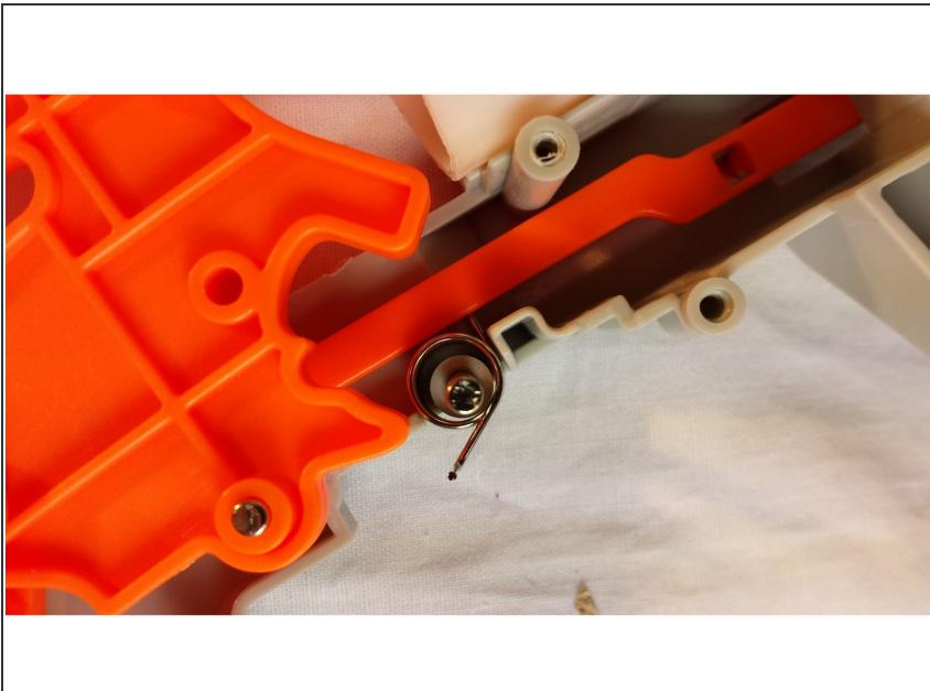
ⓘ A second set of hands would be useful during this step. Make sure the orange slide is above the spring.
