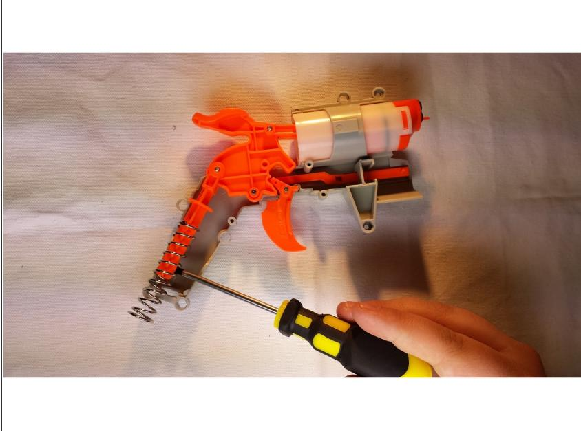
⚠ This is where the spring load mechanism is located, be cautious not to damage. If the spring separates from the gun, reattach it using a screwdriver end.
