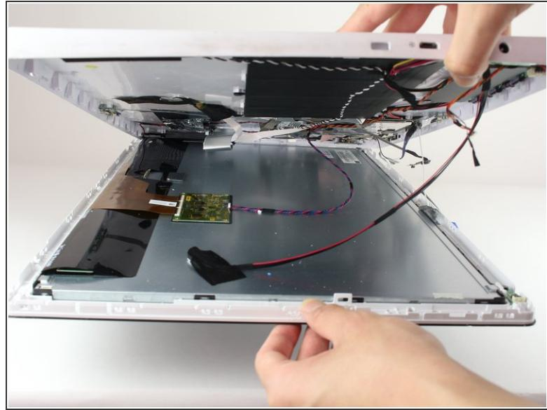
★ Flip the device over so that the back assembly is facing you.
