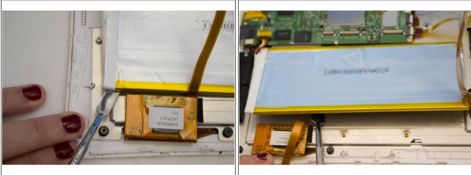
**⚠** These images show the use of a metal spudger. Use a plastic card or opening pick to avoid puncturing the battery.
