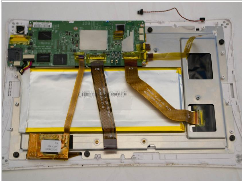
*(i)* Before removing the battery, be aware that it is held together by a strong adhesive. The battery itself is very malleable and flimsy, so make sure to handle it with care.
