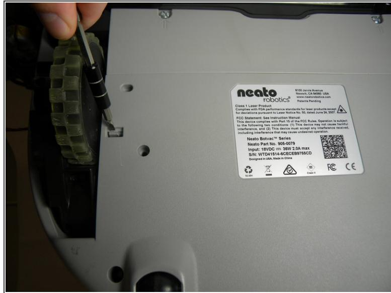
⚠ Flip the botvac over being careful not to drop the IR sensor or cause damage to the wires.
