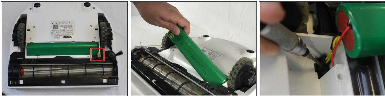
**⚠** Be careful when taking out the battery. Do not pull on the wires or battery trying to get the connector out.
