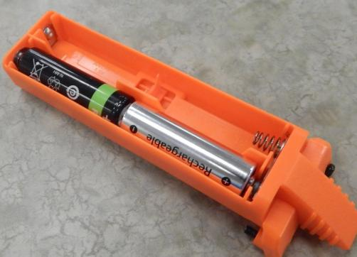
ⓘ When installing new batteries, ensure that their polarities are facing the correct directions. Follow the inscriptions on the bottom of the battery tray, or place the flat side of each battery against the spring.
