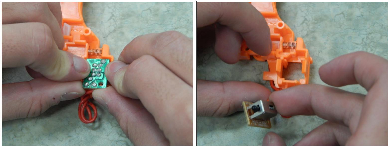
⚠ The circuit board has sharp metal solder points on it. If your finger slips you could injure yourself. Consider using gloves.
