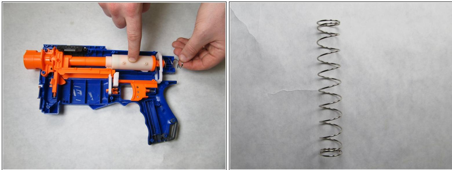
⚠ The spring may be compressed. If so, carefully release spring pressure before proceeding.
