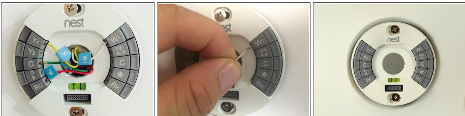
★ Remember to turn off the power to your HVAC system and the thermostat.
