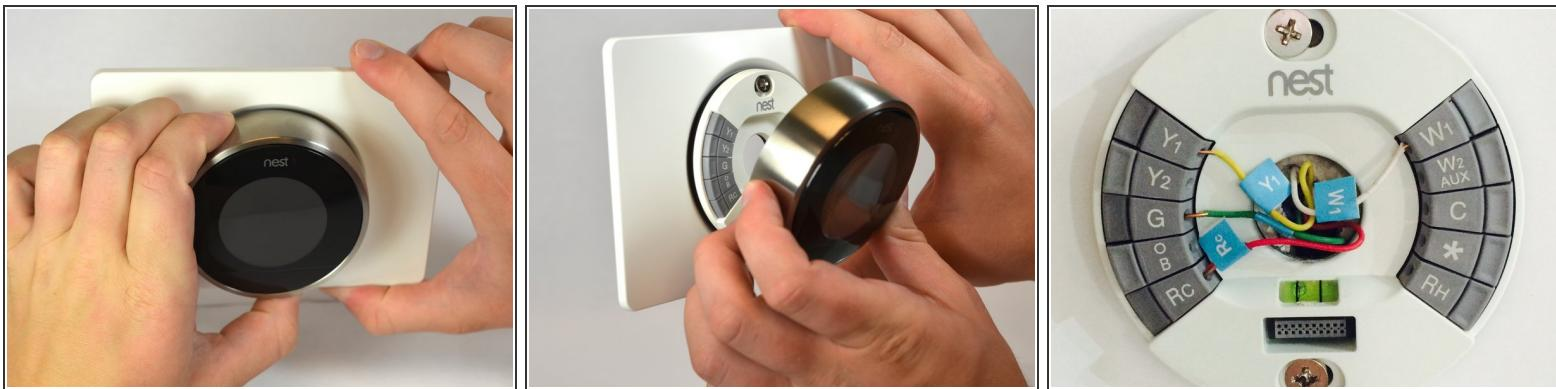
! Before disassembling your Nest Thermostat, be sure that your HVAC system is powered off.
