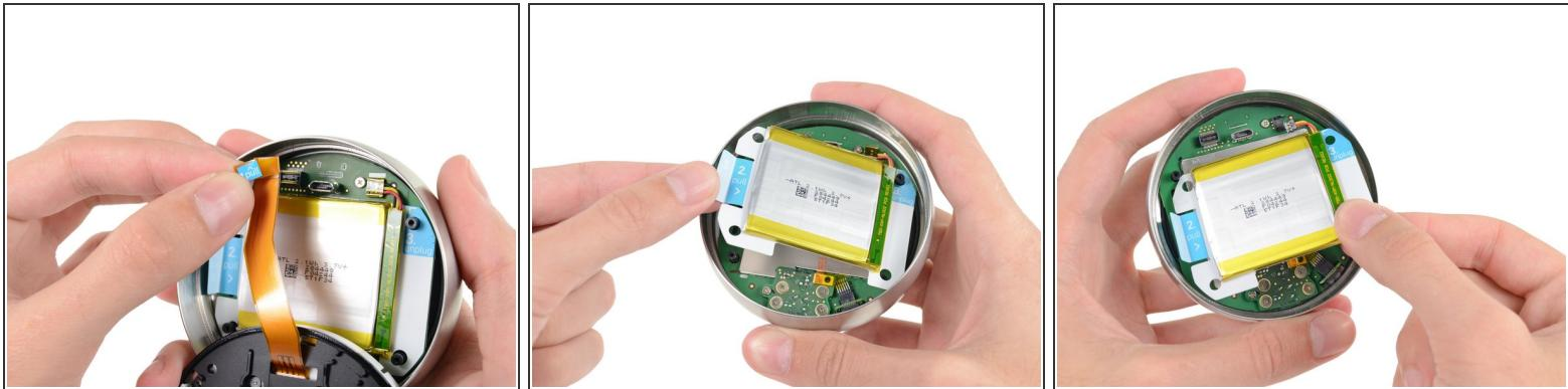
ⓘ Nothing makes us happier than a device with an [easily replaceable battery](#). We feel the engineers at Nest Labs must have been thinking of us when they added these numbered flags showing three easy steps for battery removal.
