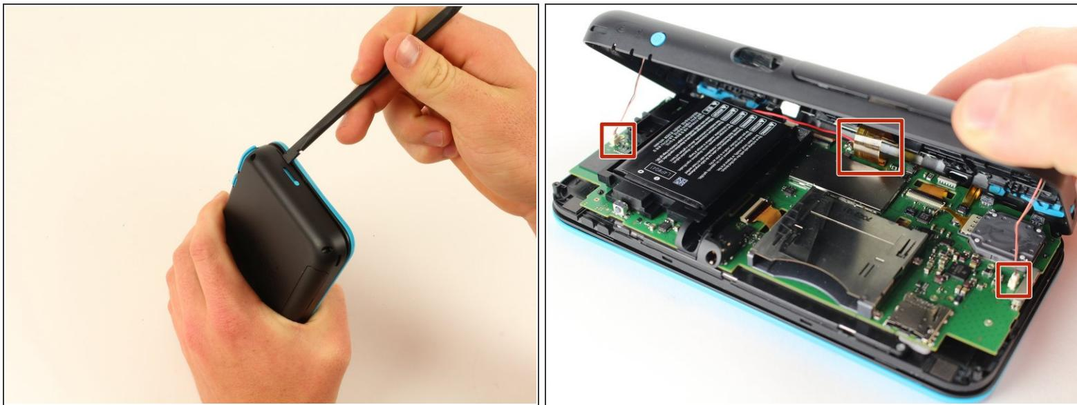
⚠ Be careful when separating the bottom panel from the front casing to avoid breaking the three cables connected to the motherboard (two on each side and one in the rear).
