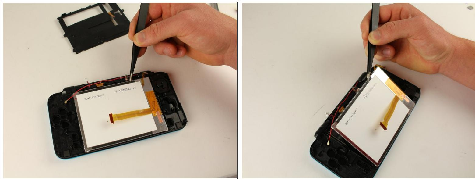
**⚠** The bottom screen is stuck to the front with an adhesive border. Be careful to slowly separate the two. Quick separation can damage both components.
