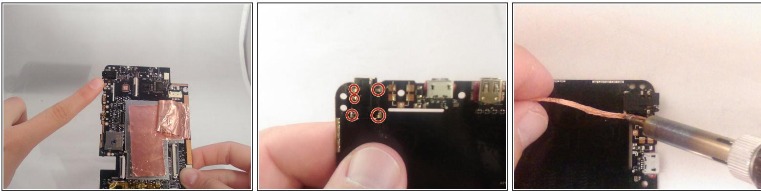
**⚠** Please review the following link for instructions on how to use the soldering equipment to de-solder properly: [Soldering Skills](#).
