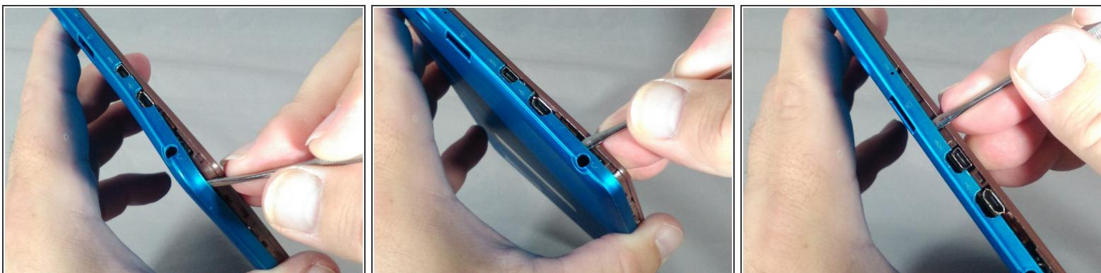
! Be careful once you get to the top of the tablet with the spudger so as not to damage the headphone jack and other ports.
