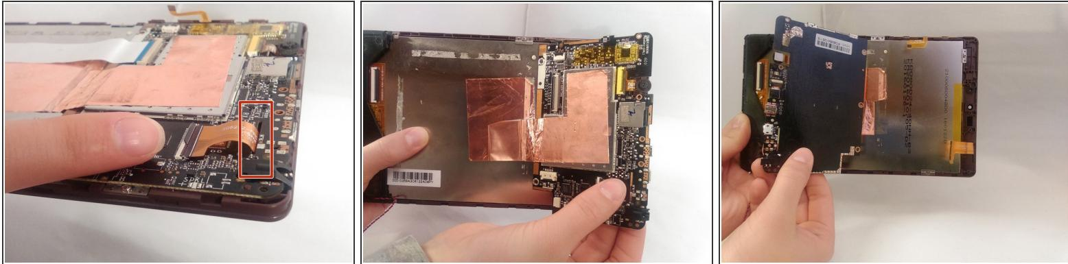
**⚠** Ensure the ribbon cable does not get caught when removing the motherboard. Damage to the ribbon cable may result.
