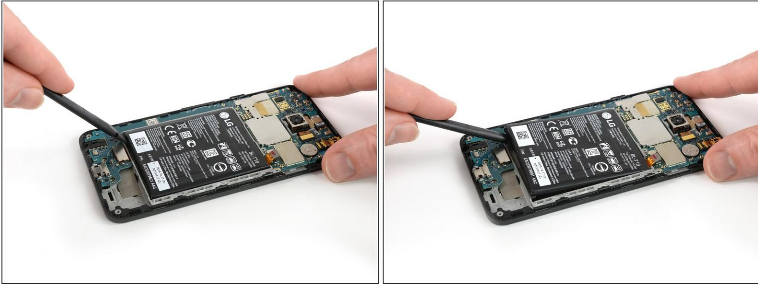
**⚠** Try your best not to deform the battery during the following removal process. Soft-shell lithium-ion batteries can leak dangerous chemicals, catch fire, or even explode if damaged. Do not use excessive force or pry at the battery with metal tools.
