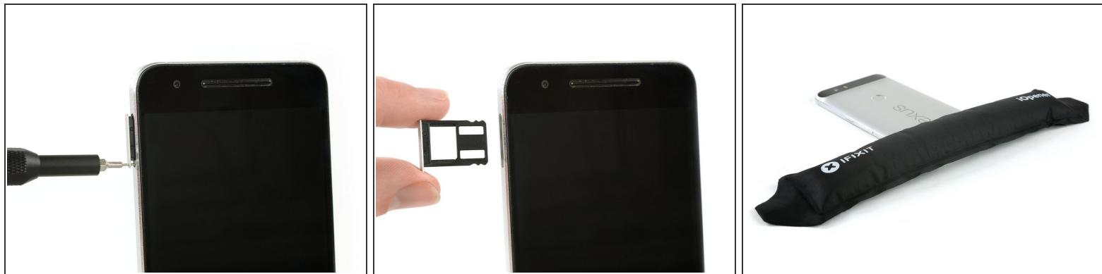
**⚠** It is possible to remove the back cover with an iOpener as seen in this guide but it's a lengthy and difficult procedure. We recommend a heat gun or something similar. The adhesive in the Nexus 6P is extremely sticky and especially the glass and plastic cover on the backside break or bend most of the time whilst doing this repair.
