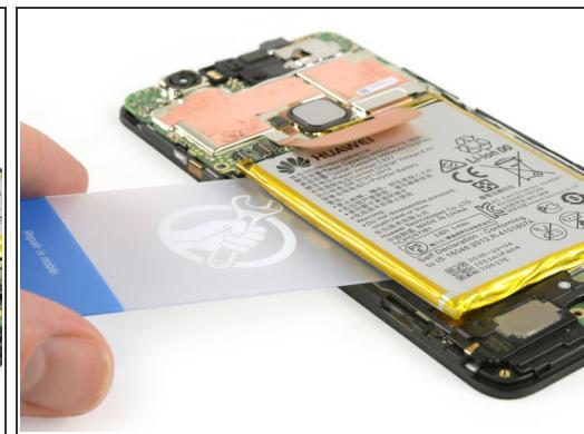
! **Warning:** do not insert the spudger or plastic card too deep underneath the battery. The display cable runs underneath the battery.
