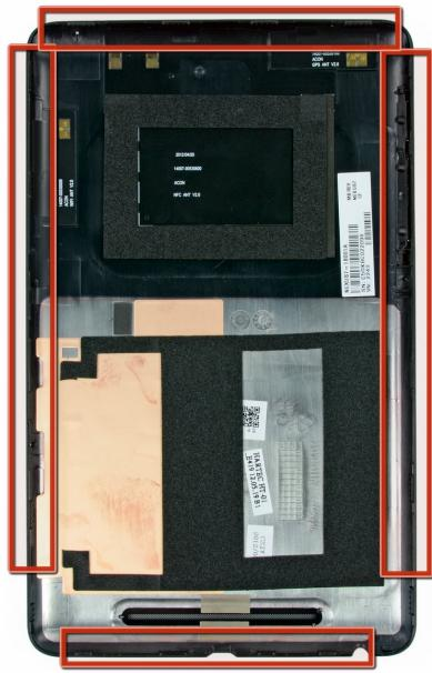
*(i)* In the following steps you will release the clips (highlighted in red) along the perimeter of the Nexus 7's rear panel.
