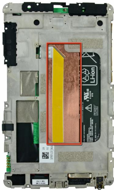
**i** The display assembly is held in place by a large amount of adhesive on the underside of the large copper ESD shield. In the next few steps, you will be using a plastic spudger to release this adhesive.
