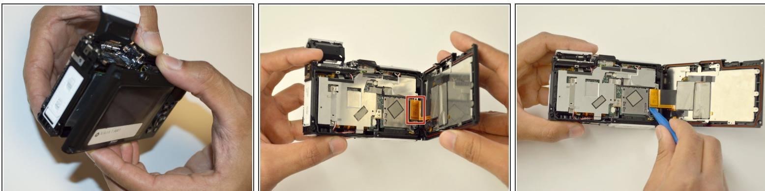
! Separate rear panel from the camera main body, starting from the HDMI and USB connector side. Do NOT pull the rear panel completely off of the camera yet.
