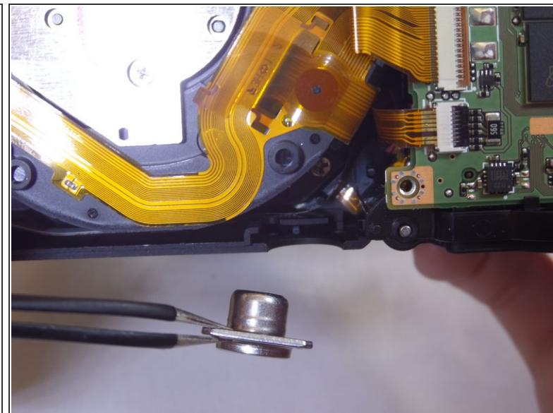
ⓘ The tripod connector is located at the bottom of the camera.
